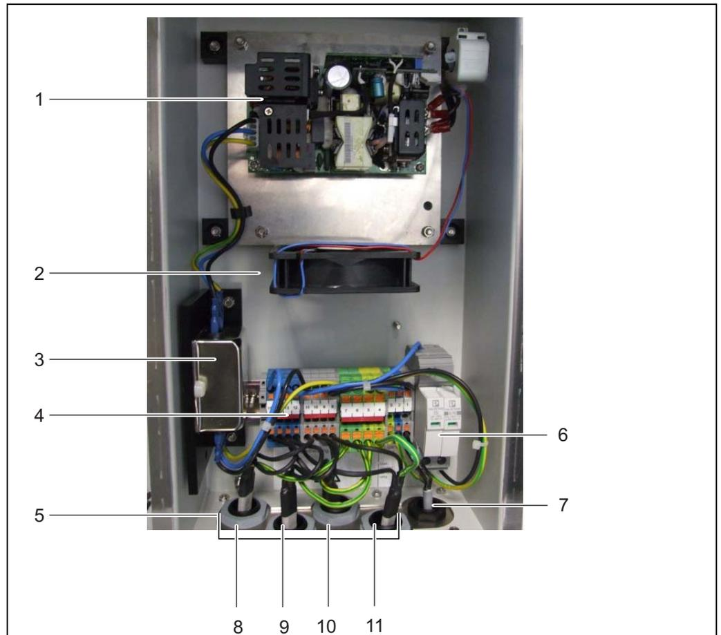
figure 3-23 Connections of the power supply box
