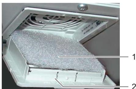
figure 5-16 Exchanging the lower filter mat
