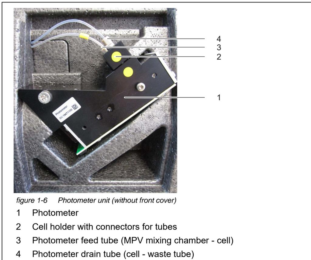
figure 1-6 Photometer unit (without front cover)
