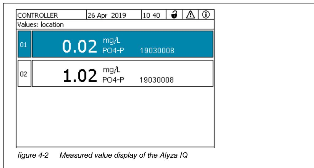
The current Alyza IQ measured values are also displayed in the Alyza menu, tab *Status*. More detailed information on the current status is available here, (e.g. next measurement, next cleaning, next calibration).
