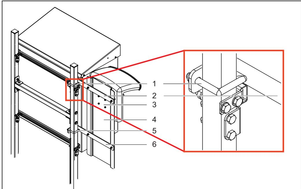
figure 3-19 Installed terminal holder TM (view of the rear side)
