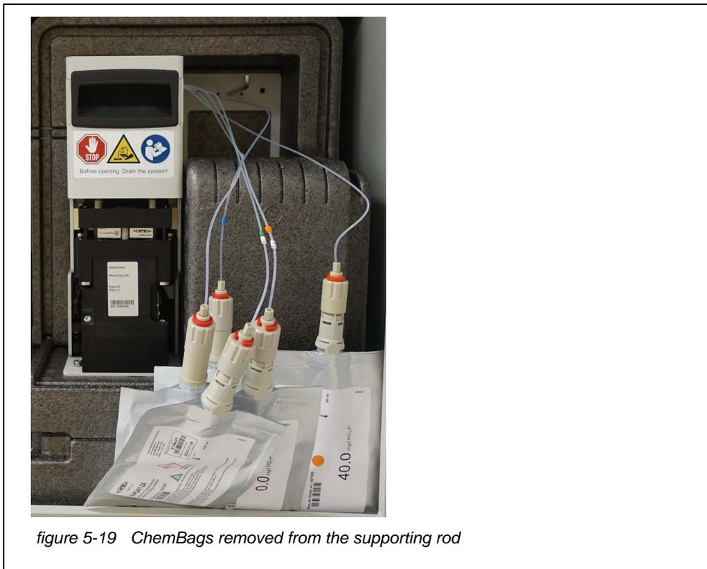
figure 5-19 ChemBags removed from the supporting rod
