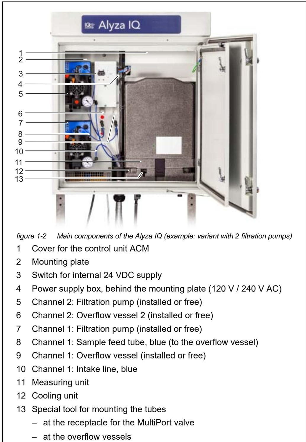
The measuring unit ready for operation (11) includes the following components
