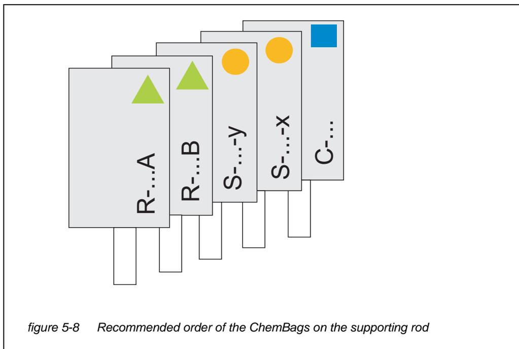
figure 5-8 Recommended order of the ChemBags on the supporting rod
